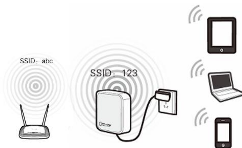
Figure 2-4 Hardware Installation of the TL-WR702N in Bridge Mode
