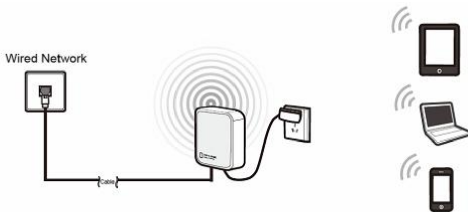
Figure 2-1 Hardware Installation of the TL-WR702N in AP Mode
