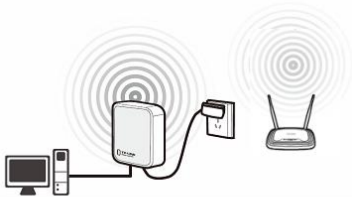
Figure 2-5 Hardware Installation of the TL-WR702N in Client Mode
