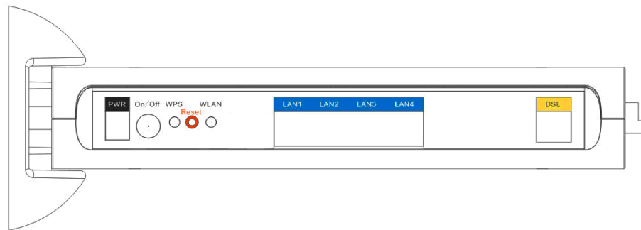
FIGURE 2 REAR PANEL INTERFACE DIAGRAM
